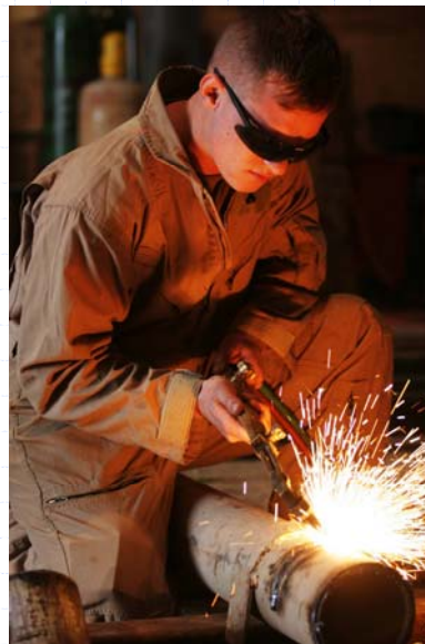
Manual oxy-fuel cutting
