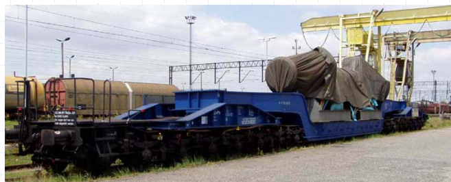
Heavy transport on railway, capacity of the car is 120 t
