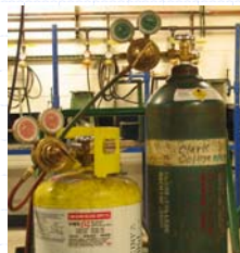
Compressed gas cylinders containing oxygen and acetylene gas
