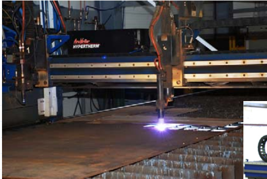
Automatic oxy-fuel cutting
