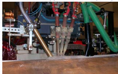
Submerged arc welding
