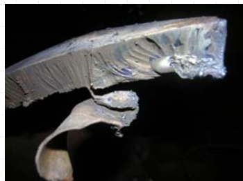
Edge of steel plate after oxy-fuel cutting
