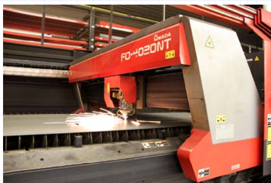
Industrial 4kW laser with flying optics system
