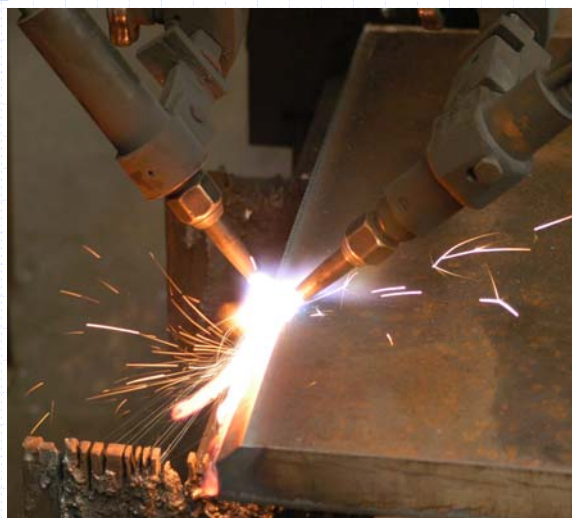
Preparation of edge for butt weld of thick plate by oxy-fuel cutting
